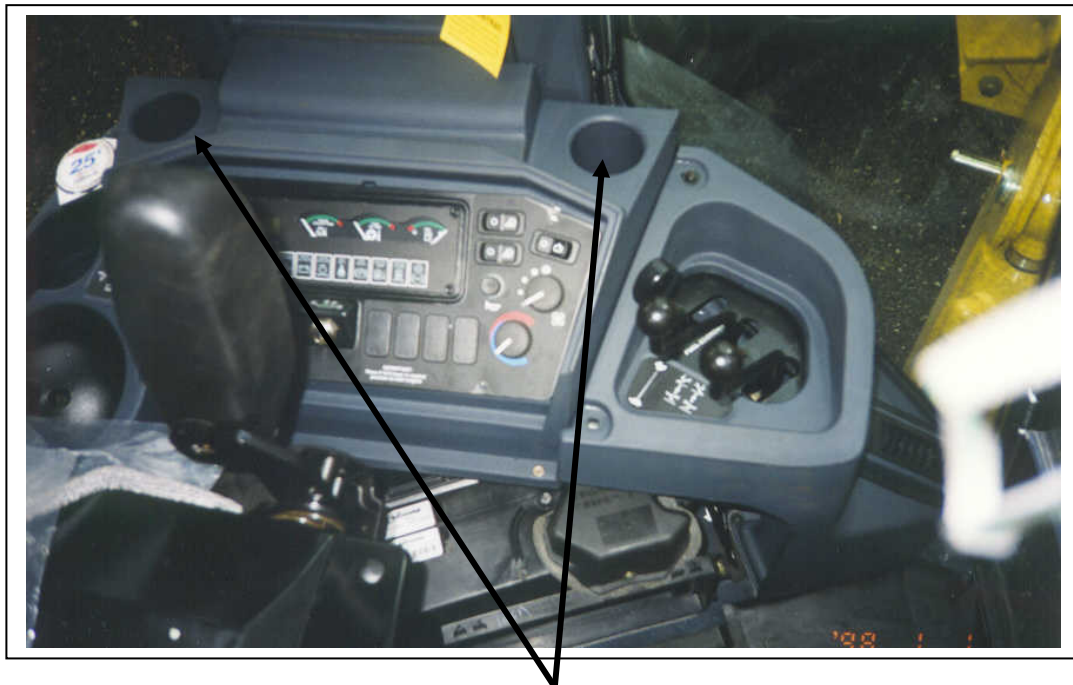
Vent can be installed in either cup holder location.
